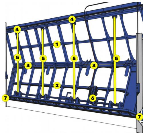
A bifold door is a two-piece system: a top panel and a bottom panel hinged together in the middle. Bifold doors typically include:
